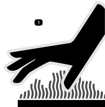
1. Hot surface (on exhaust baffle)
